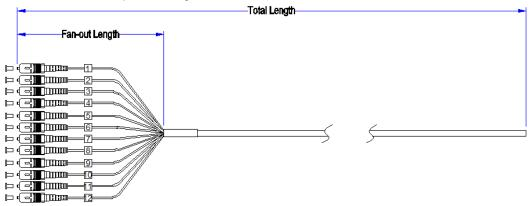
Pre-terminated Indoor Cable System with Single Staggered Fan-out
